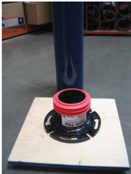
Figure 2. The second method for building a cane stand, using a toilet flange.
